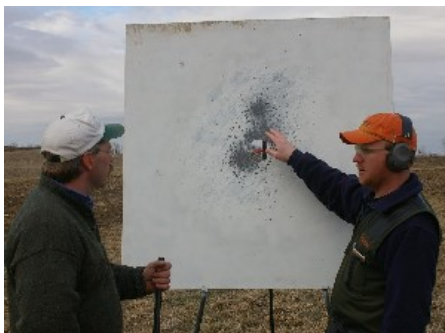
Fit evaluation at the pattern plate shows where the gun is shooting in relation to where the shooter is looking
